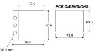
Flange mounted enclosure to be used for thermostats, relay boxes etc. PCB and packing are available.
