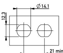
See product drawing or recommendations for use the M12 90° connectors together with housings which have already an integrated M12 thread (**ERNI document 225406**).
