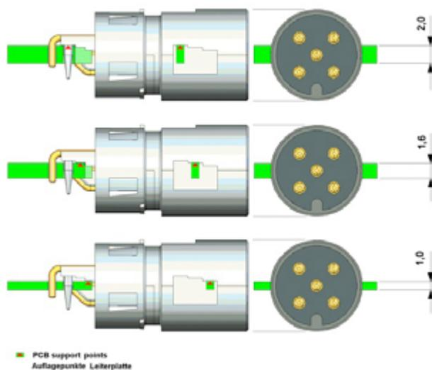
The connector has integrated PCB support points, which are able to adapt the 3 frequently-used PCB thicknesses. The thickest PCB could be 2.0 mm followed by the favorite 1.6 mm and further followed by the thinnest 1.0 mm.
